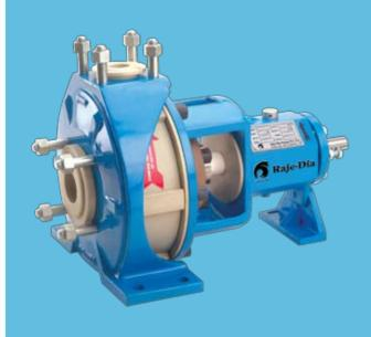
Series 'RD' pumps are a variation of series 'PPE' pumps which incorporate back-pull-out feature. This offers all the advantages for easy maintenance, similar to metallic pumps. The metallic armour supports piping loads without any strain on the pump suction and discharge nozzles.
