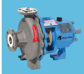
Series 'AER' metallic pumps are designed for heavy-duty service with oversized bearings for reliable operation. The Robust semi-opened impeller design handles moderate percentage of solids without clogging. The sturdy shaft design minimises vibration and provides smooth & trouble free operation. The pumps are offered in various materials like Carbon steel, SS 304 (CF8), SS 316 (CF8M), SS 316L (CF3M), A-20, Hast-C, Hast-B etc.
